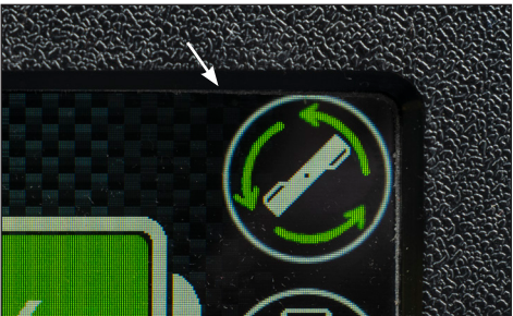
fig. 3E – Blade Speed icon on the operator touch screen.
