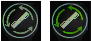
Blade Speed Low (Grey) / High (Green) Indicates the speed of the blades during operation.
