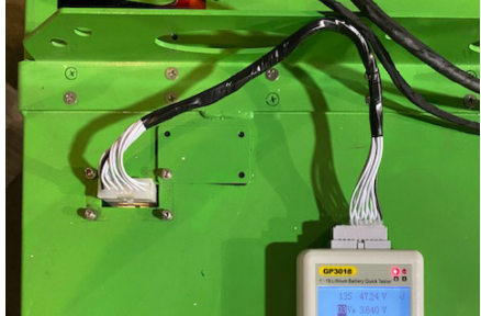
fig. 1C – Handheld tester connected to the port on the battery.
